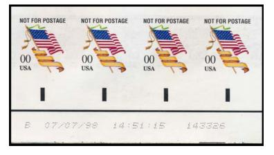
This bottom margin strip of four (cropped from the portion of the web section shown on page 2) shows the inkjet marking (B 07/07/98 14:51:15 143326) that was applied once per revolution of the gravure cylinders. This indicates these test stamps were printed at 2:51 PM on July 7, 1998 and that the counter had recorded 143,326 plate impressions (it seems likely the counter hadn't been reset at the beginning of this press run).
