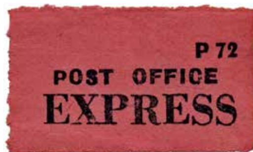
Fig. 3. Enlargement (3.5×) of the label in Fig. 2(b) shows paper-fiber characteristics and indeterminate borders.
