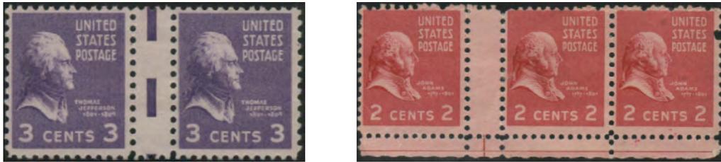
Gutter pairs represent a total failure of the production and inspection process. Horizontal or vertical gutter pairs can exist showing the common margin between two adjacent panes that should have been trimmed down the middle to create two separate panes. The basic cause is simple – the failure of the cutting process to separate two sheets in the appropriate manner.
