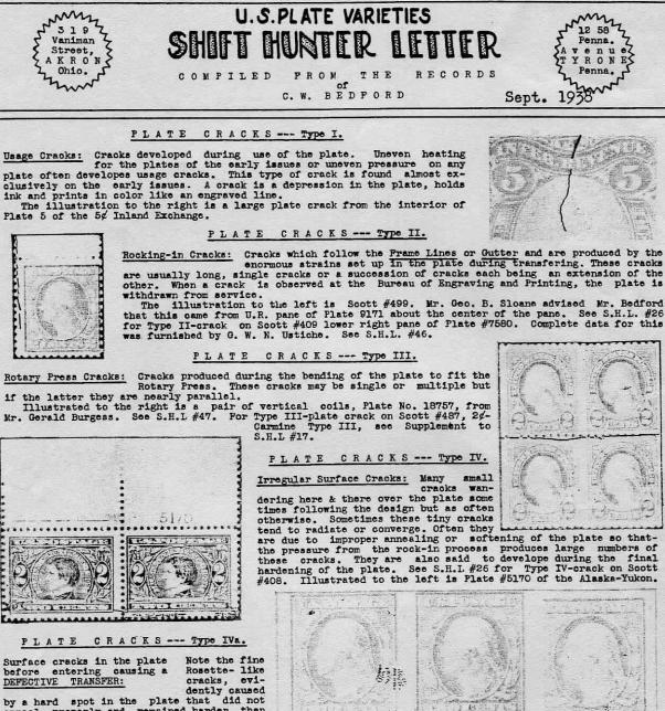
by a hard spot in the plate that did not anneal properly and remained harder than the rest of the plate. When the stamp was rocked-in over this crack the metal was so hard at this spot that the right frame line of the design did not transfer properly .... This left what we call a Defective Transfer (See Supplement to S.H.L. #17.)
