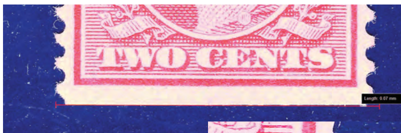
Figure 2. The typical screen image (above) shows that this specimen's edges are not parallel.
