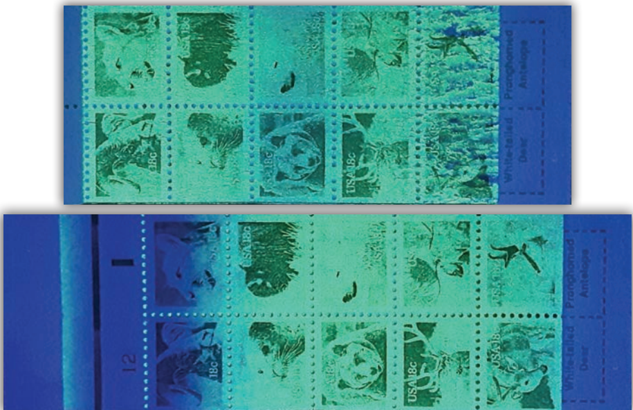
Figure 6. Tagging mat deterioration in a plate number 12 booklet.
