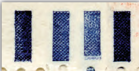
Figure 7. Engraving of the length register marks (LRMs) on plates 1 at (left) to 4 (at right).
