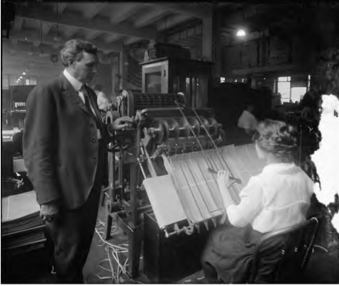
Figure 10: Early model of a 2-way rotary perforator. Web alignment controlled by two operators.
