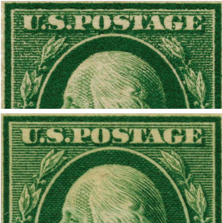
Figure 3. Eroded plate at top, fresh plate on the bottom.
