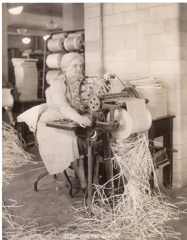
Figure 9 (above). Auto-Wound stamp coiling machine (image courtesy of Mick Hadley).
