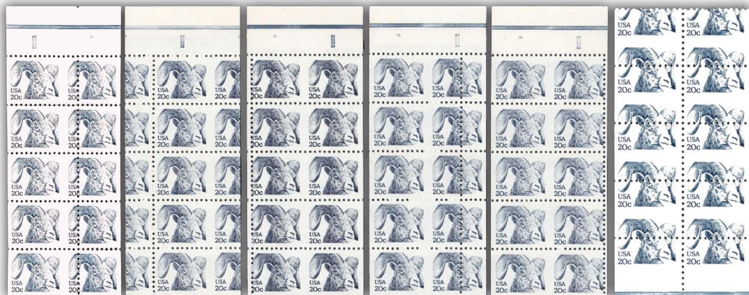
Figure 7. Typical misperforations and miscuts in BK142.
