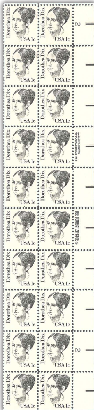
Figure 22. Plate strip from sleeve two showing electric eye marks added to accommodate the L perforator.
