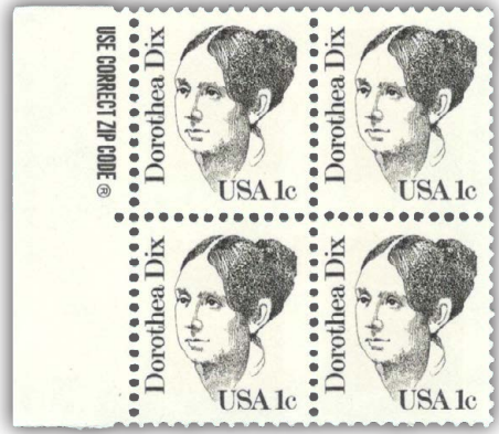
Figure 14. Bullseye perforations produced by the A Press integral perforator.
