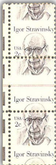
Figure 11. Miscut shows the joint lines that fill with ink between plates.
