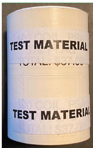
TD138 - Two connected unopened coil rolls of 100. The "TEST MATERIAL" label is 1-3/4" x 1/2". Coil roll is 1-3/8" in diameter. Separations are serpentine die-cut gauge 10-1/4.
