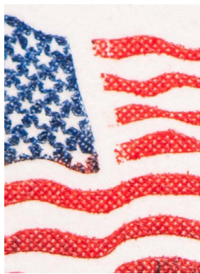
Figure 11. The genuine intaglio printed stamps have raised, well-defined details.
