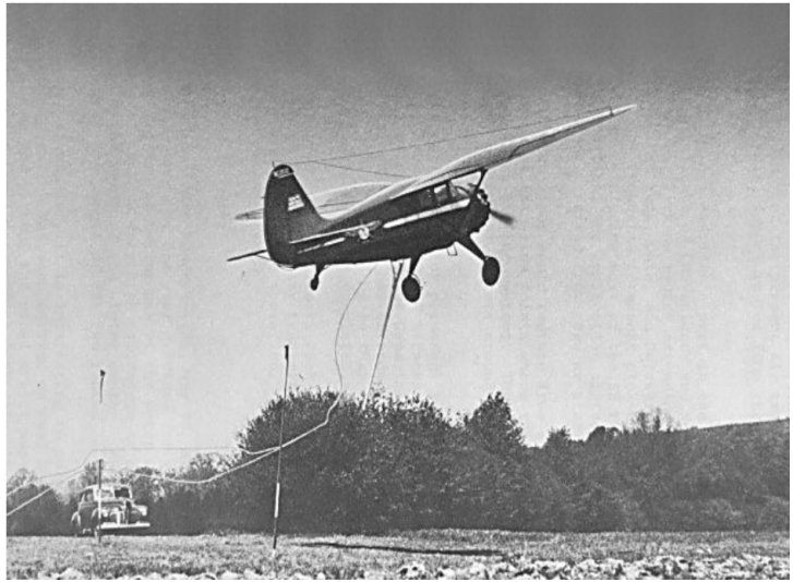
Figure 11. Stinson Reliant aircraft swooping down to snatch a mailbag suspended on a rope between two poles.
