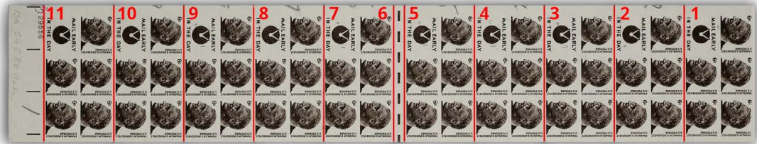
Figure 8. Locations of the final knife cuts on a strip of booklets.
