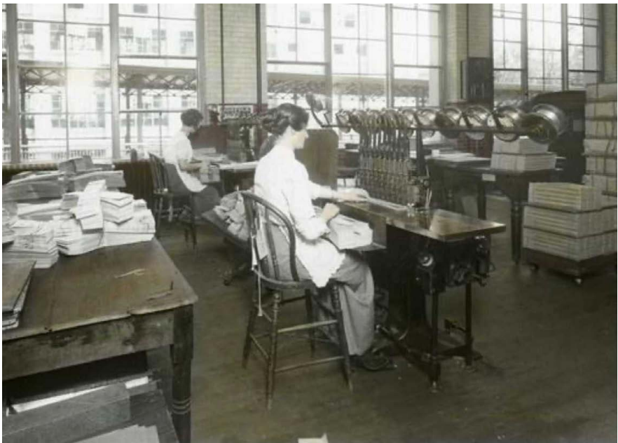
Figure 7. Ten-Head stitching machine, ca. 1910–1920.
