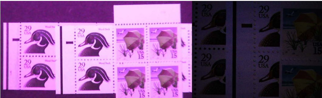
Figure 5. Long-wave UV image from the Panasonic camera and Tomlov microscope, both set to automatic.
