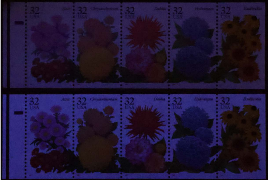
Figure 10. Dead and high bright paper under long-wave UV illumination.
