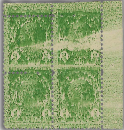
Figure 2. FBI Rotary sheet-stamp "start-up spoilage," over-wetted paper, plate wipers inactive, ungummed; perforated later on the Stickney two-way perforator while still on the web roll.
